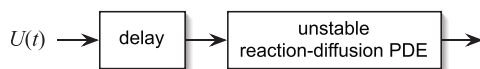
Fig. 7. Control of an unstable parabolic PDE with input delay, that is, of a boundary controlled cascade of a transport PDE and a reaction-diffusion PDE. Explicit gains are derived for the predictor feedback (83). As stated in Theorem 8, stability is achieved in a somewhat non-standard Sobolev norm, rather than in the basic L_2 norm of the state of the PDE cascade.
