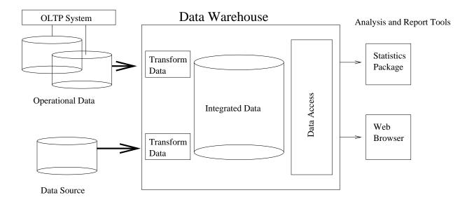
Figure 1: Data Warehouse Architecture.
